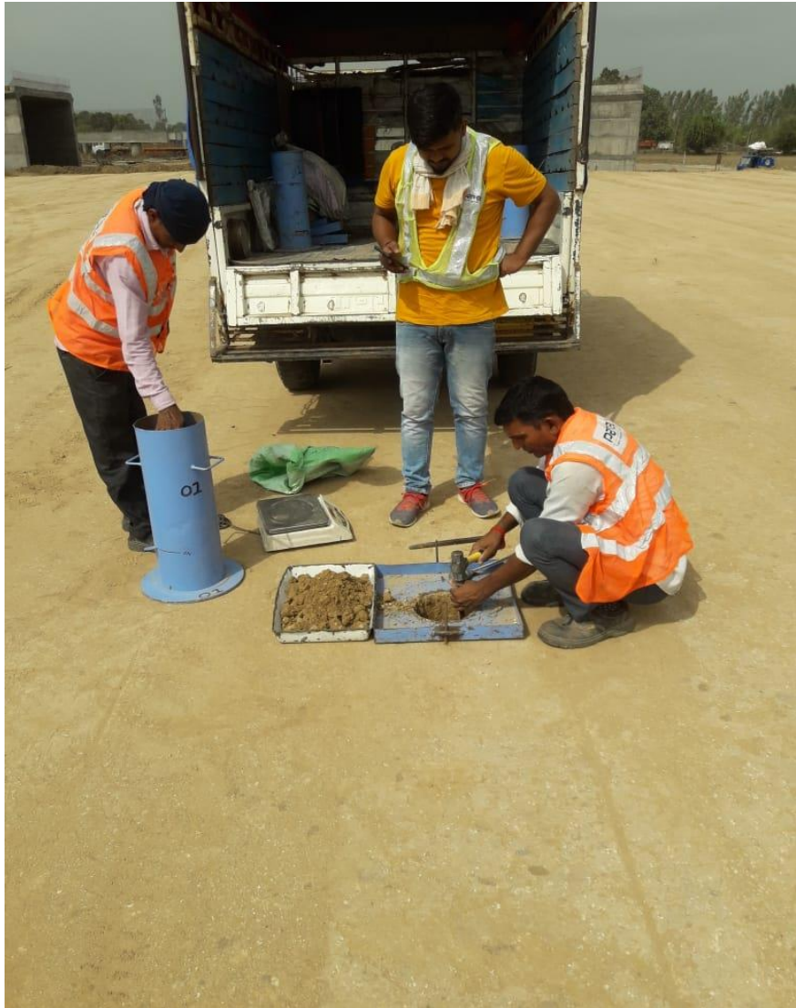
FDD checking at Project Site
